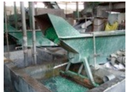
Flake from grinder to float/sink tank
